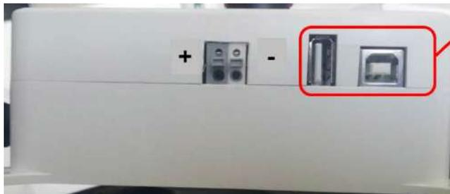
Daisy chain PVG-C w/ USB cable. USB type-B (square) is the starting point, and USB type-A (flat) is the ending point. BDG-256 is the starting point if connected.
