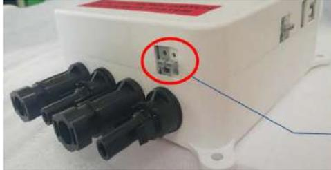
Connector for external PLC signal ring
