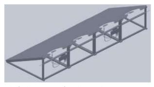
Once the final position is confirmed, secure the microinverters using the MLPE clamps and torque per the manufacturer's specifications. Typical values are about 12 ftlbs (16.3 NM).
