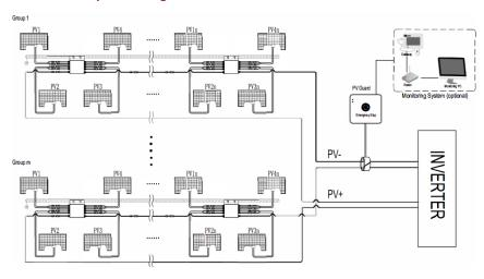
Port PV-1 must be connected to a PV panel to power the PVG.Cables (PV+ and PV-) of an unused PV port shall be connected.
