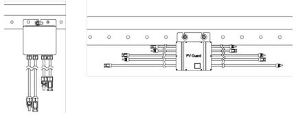
If the PVG is mounted at the back of a PV panel, installer shall follow PV module installation instructions. The minimum distance betweenany portion of PVG to the back of the PV panel shall be at least 0.5 in.
