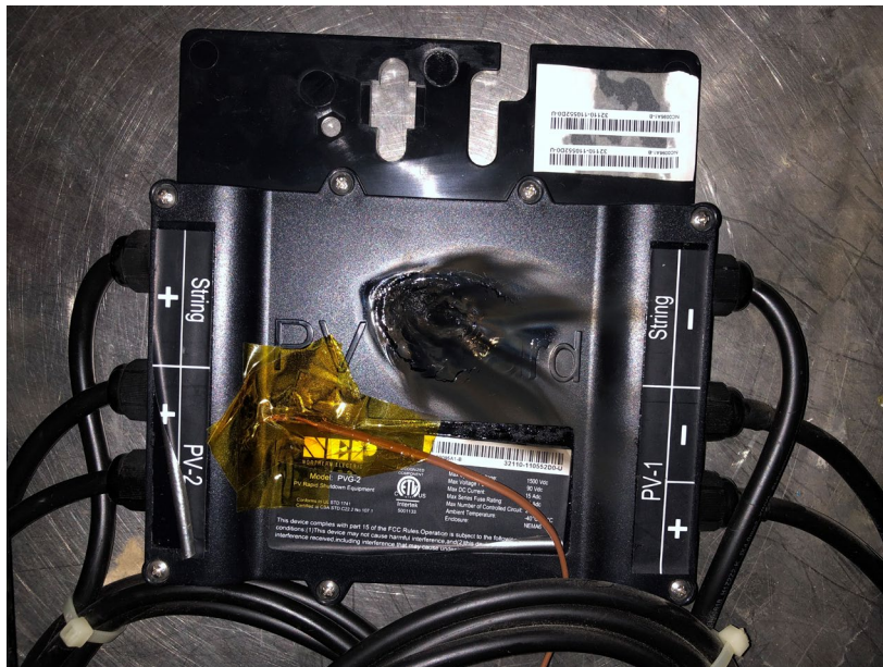
Figure 3-11: RSD Enclosure Once Flame Source was Removed
