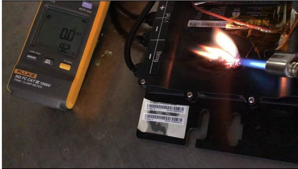
Figure 3-10: Flame / Burn Test in Progress
