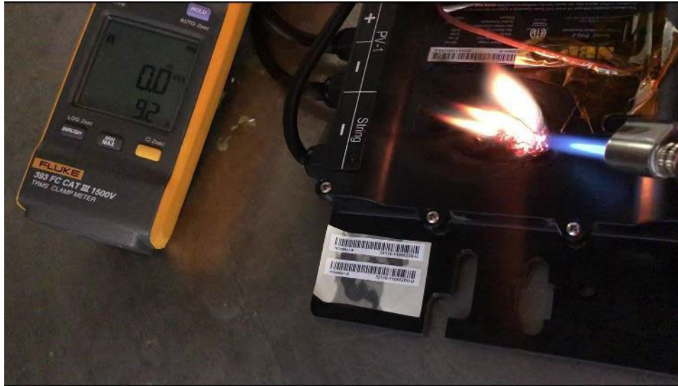
Figure 1-3: Flame / Burn Test in Progress
