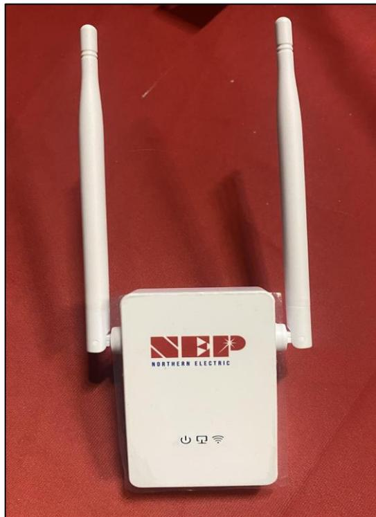
Plug in Booster near router, and connect an ethernet cable between them.
