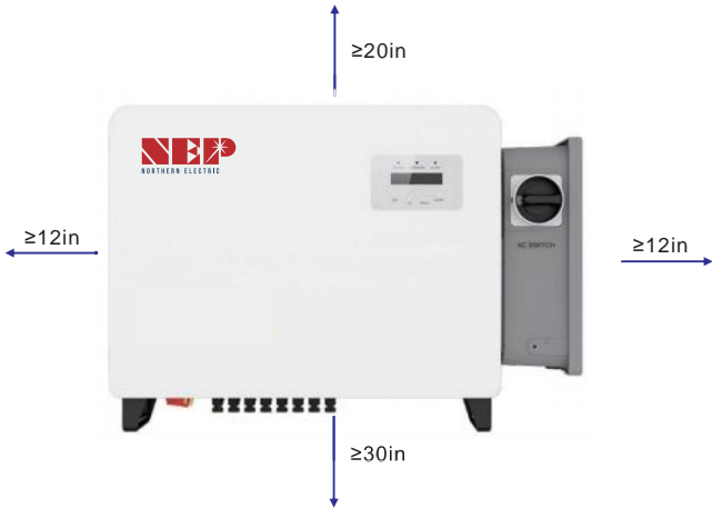
Figure 3.2 Clearance distances requirement for the inverter
