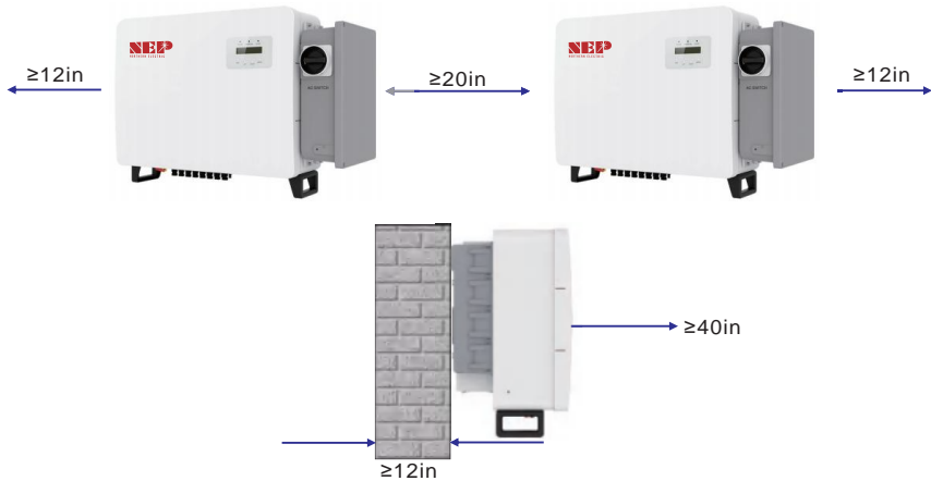
Figure 3.3 Distances required between inverters when multiple inverters are installed
