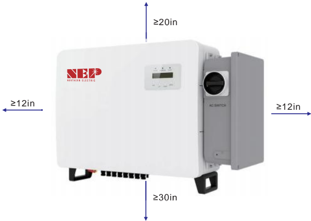
Figure 3.2 Clearance distances requirement for the inverter
